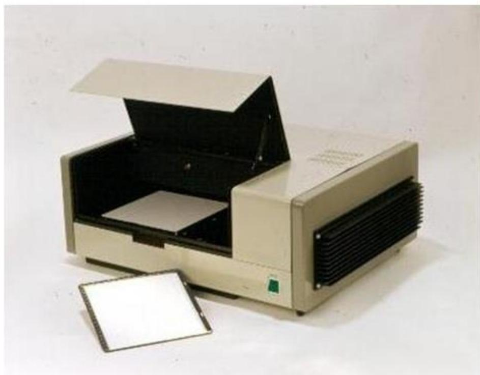
10. Spectrofluorometer, Quanta master 40
