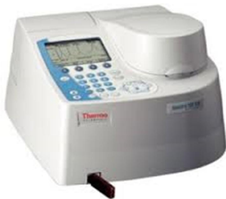
Spectrophotometer UV-VIS GENESYS 10S
